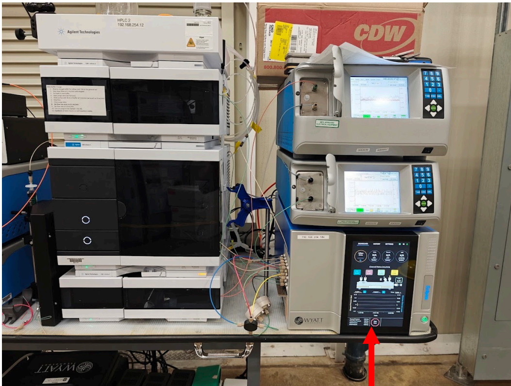
Wyatt Eclipse integrated into HPLC-SEC-MALS stack
